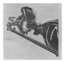
FIG. 5 -- KNUCKLE OIL SEAL
